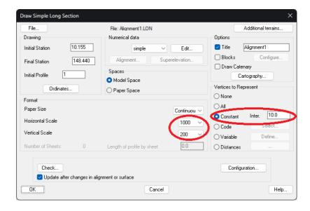
4. Click OK to draw the longitudinal profile in model space and choose an insertion point in a clear area of model space.
