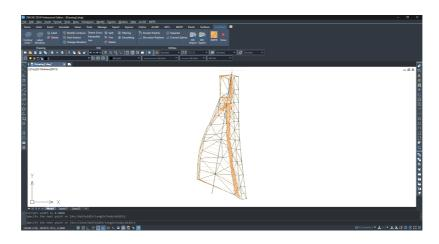
2. Run MDT9 > Horizontal Alignments > Convert Polyline to Alignment and select the previous polyline
