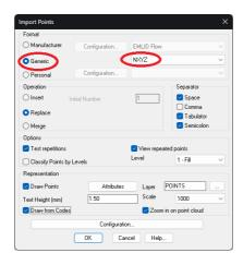
4. Choose a suitable Scale for the representation of the texts and uncheck the Draw from Codes option.
