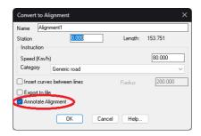
3. Enable the Annotate Alignment option and click OK two times
