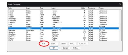
2. Select the item from the list to be modified and click the Edit button. The figure shows the LS code (Low Slope) which is of type Line and will be drawn on layer LOW\_SLOPE in Magenta color.
