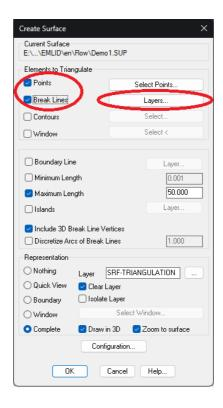
3. Choose the list of layers that should be considered as break lines, drawn automatically or manually, using the > button, and press OK
