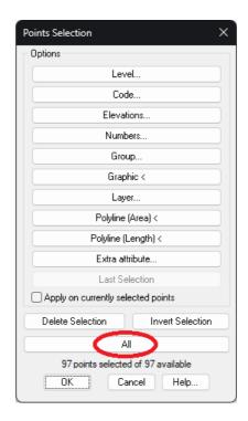
8. Press the All button and check that the point codes have been converted correctly. The ones with point geometry (e.g., TREE) appear as is, and the linear geometry ones are completed with the suffixes "S" for Start and "E" for End.
